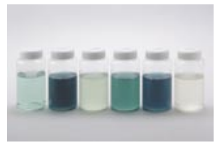
Positive samples in natural light Coliform bacteria produce the \beta -galactosidase enzyme, which then cleaves the synthetic substrate X-GAL contained in the ECBlue and simultaneously releases a blue/blue-green dye.
