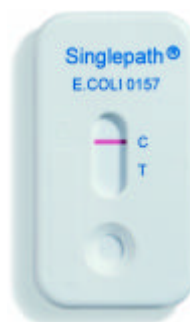
Singlepath® E. coli O157 Test result negative
