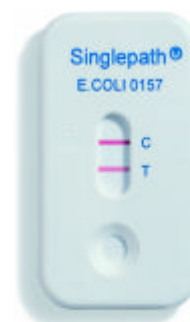
Singlepath® E. coli O157 Test result positive
